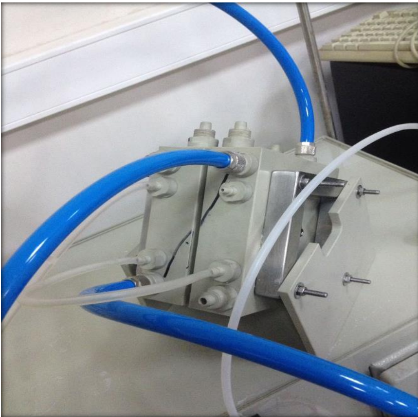
Figure 3.3 Pictures of the closed RED module
