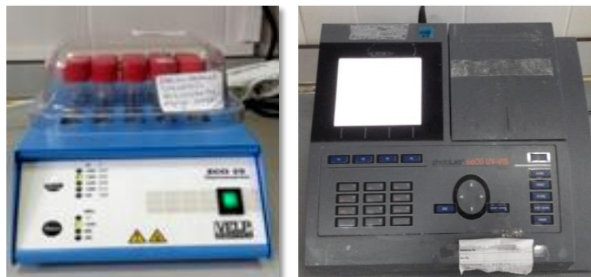
Figure 3.8 Apparatus used for COD analysis; from left to right: VELP ECO 23 Thermoreactor, 6600 UV-VIS Spectrophotometer
