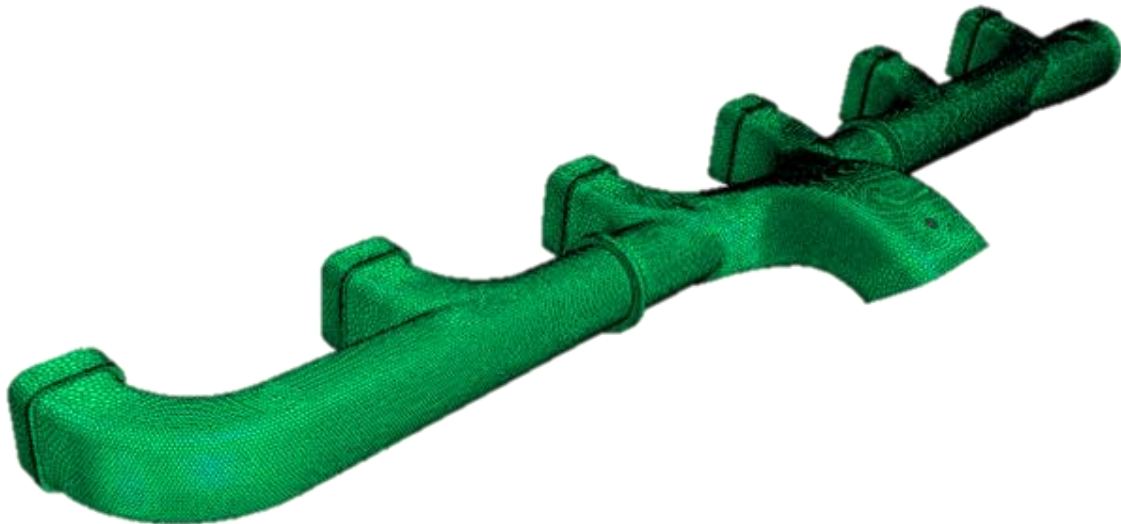
Figure 2.25 Volume Mesh of Fluid Domain at CHT Simulation
