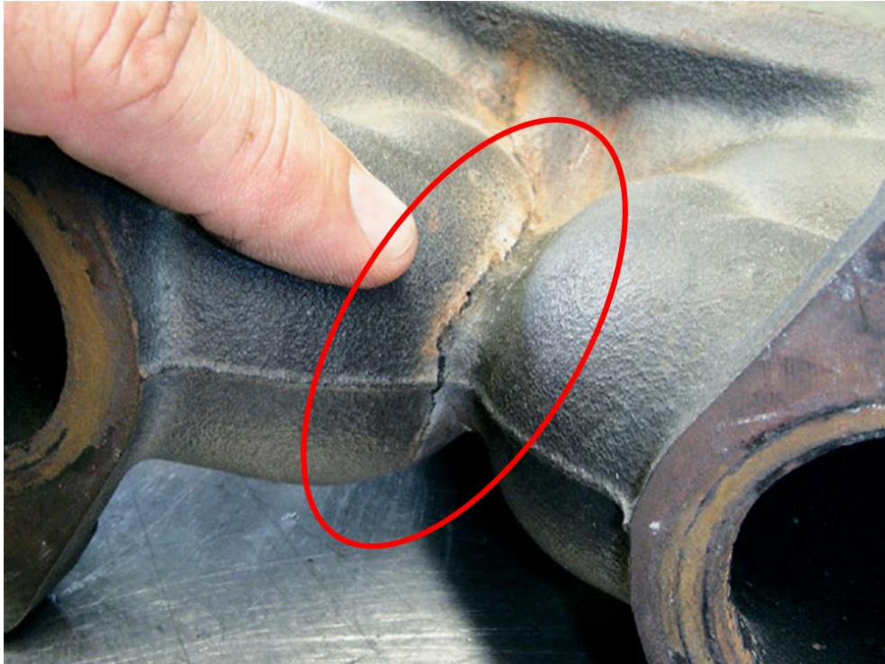
Figure 1.3 Thermal Crack on Exhaust Manifold
