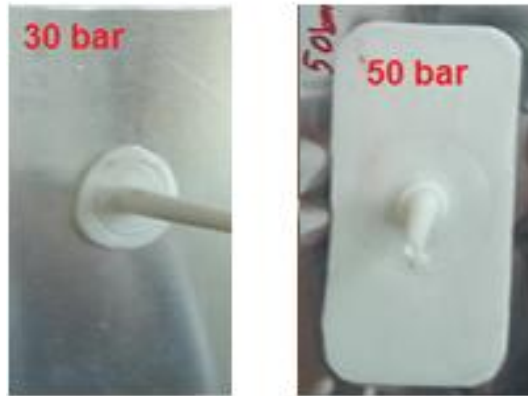
Figure 4.2 Forming limit of a 0.5 mm-thick plate through the PIF method under the influence of different injection pressures
