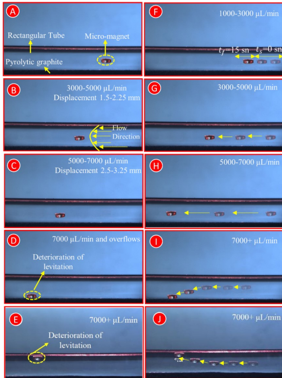
Figure 2.12. Images captured from the Point Grey microscope camera system during the experiments. Figures A-B-C-D-E display the amount of displacement depending on the flow rate. F-G-H-I-J show the applied flux-dependent and time dependent behavior of the magnet.
