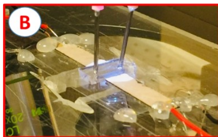
Figure 3.11 Experimental Setup of Acoustic System. The experimental setup used during the acoustic experiments are shown. The oscilloscope is used to determine the frequency at which the surface waves are generated with highest amplitude. The signal generator is used to generate a sinusoidal signal that is fed into the acoustic transducer through a voltage amplifier. Figure 3.11.A The PZT
