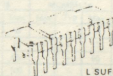
L SUFFIX CERAMIC PACKAGE CASE 680
