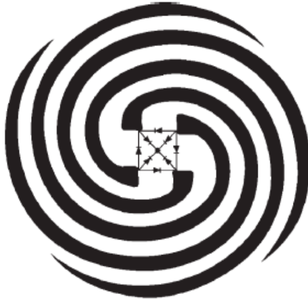
Figure 1.2 Reflectarray using a 4-arm spiral as element with switching diodes at center to achieve a 2-bit phase-shift system for circular polarization [4]
