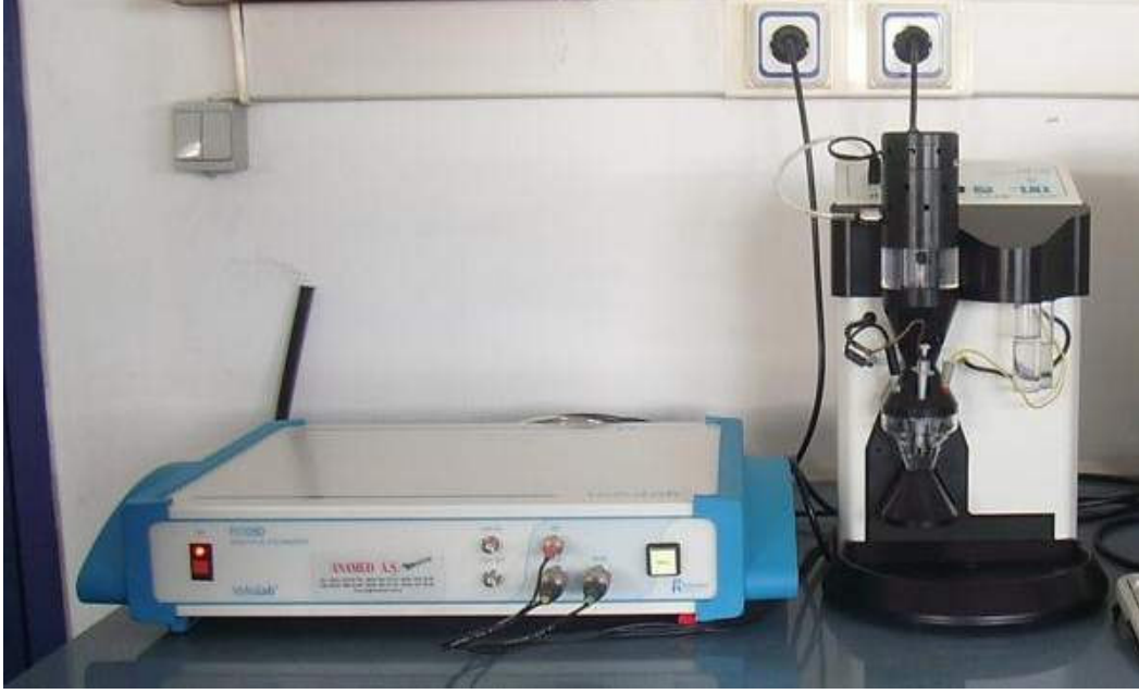
Şekil 5.2 Radiometer marka Voltalab 50 (PST050) Analitik Potansiyostat ve Radiometer marka MDE150 Polarografik Stand
