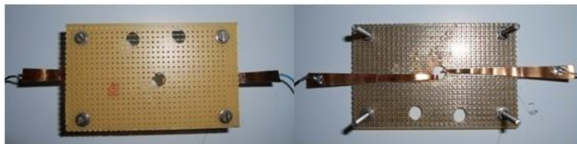
Figure 4.12 Sample stage for thin film PVs, (left) front and (right) behind
