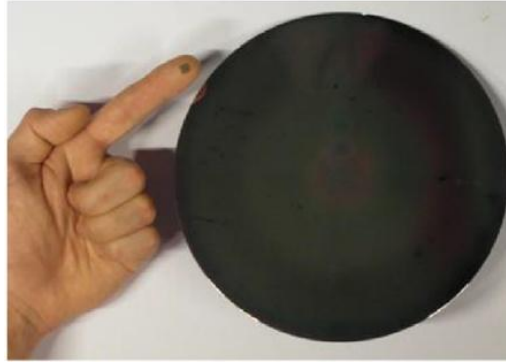
Figure 3.5 Scailing the synthesis of nanaomaterials: from 5x5 mm 2 to 200 mm wafer size [48]
