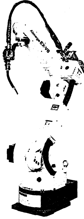
Şekil 7.2 Almega EX-MV6 ark kaynak robotu (OTC-Daihen EX Series Robot Instruction Manual)
