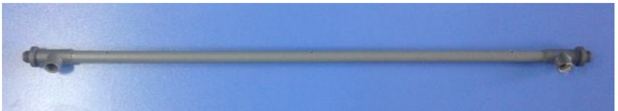
Figure 3.7 Shell of heat exchanger (test section)
