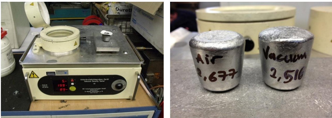
Figure 2.18 RPT Tester and Samples
