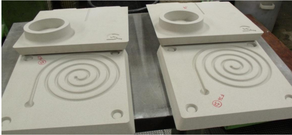
Figure 2.11 Sand spiral mold parts
