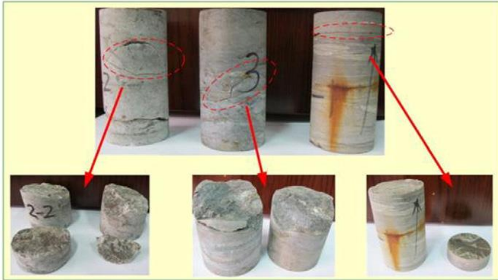
Figure 3.4 The macroscopic damage process of biotite granite under 150 F-T cycle between +40°C and - 40°C (Tan vd., 2011)
