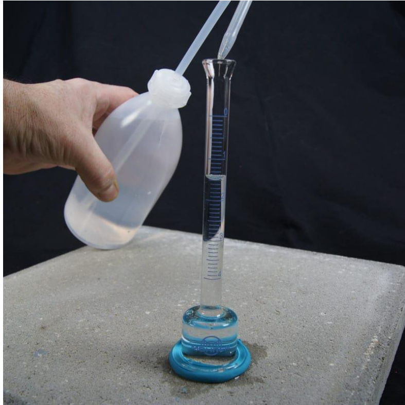
Figure 5.26 Water absorption analysis with Karsten tube
