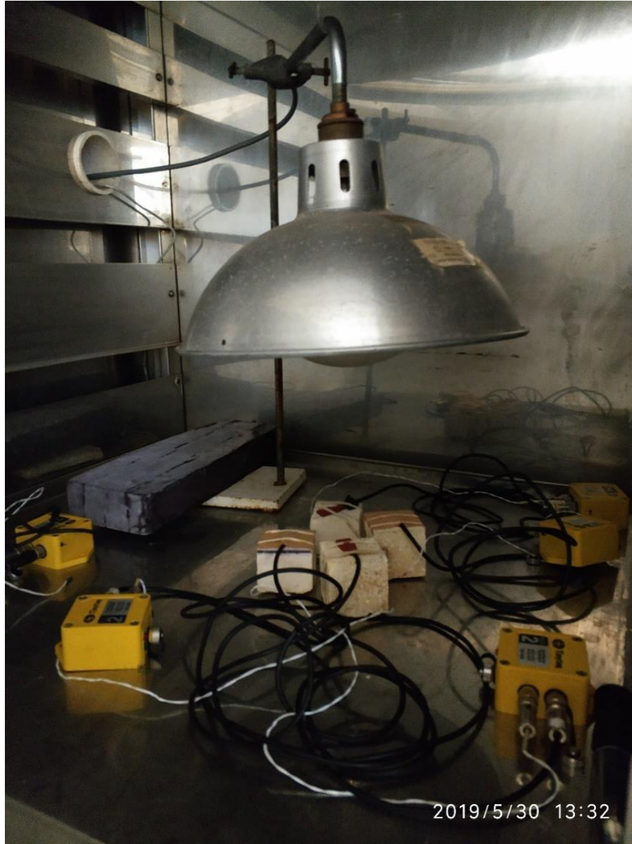
Figure 5.34 Real setup for soft capping experiment. The image shows covered and uncovered (control) samples for Mardin and Nevsehir stones. Lamp is installed about 20 cm above the stones. All soft capping experiment carried out inside the weathering chamber.
