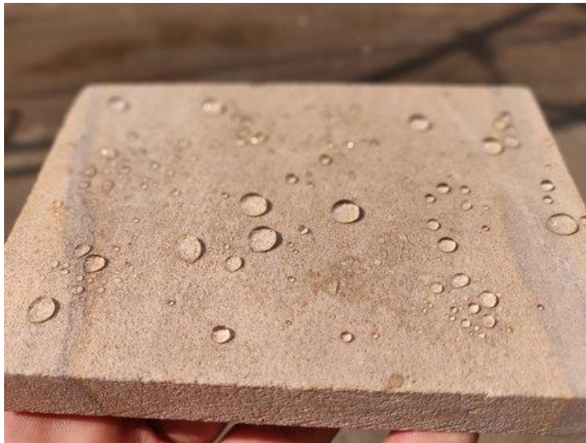
Figure 4.28 Effect of silicone base water repellent (from product sheet of Flora Metallic Flooring© TR-813)
