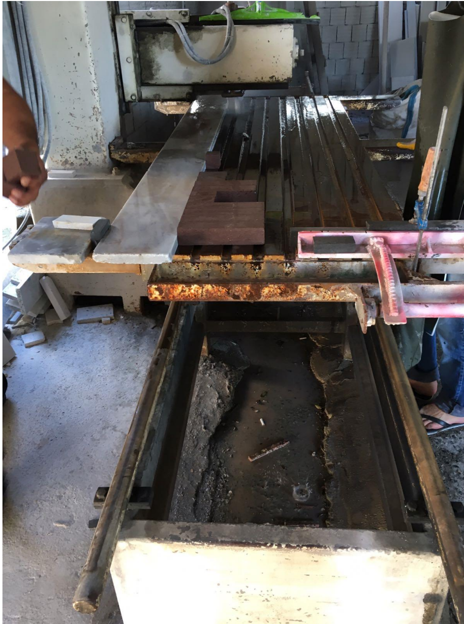
Figure 5.17 Ankara Stone is being cut by marble saw
