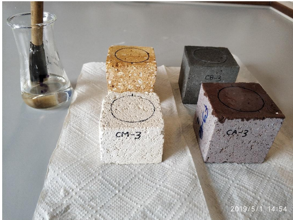
Figure 5.25 Application of DAP treatment
